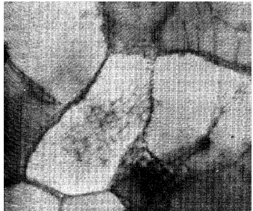
Dislocation network in cold-worked aluminum (32,500 X).
